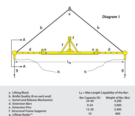
\*\* A "jumper" may also be required when lifting shorter mats. This device simply attaches to the existing lift hook and extends the length for shorter mats.
