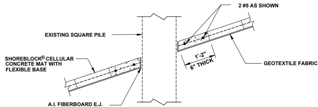
**SECTION THRU BRIDGE PILE AND CONNECTIONS**
