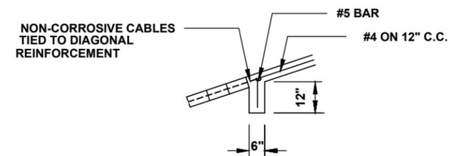
**SECTION THRU BRIDGE PILE**
