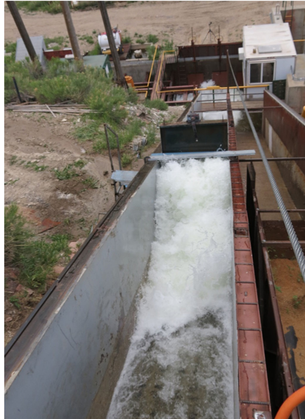
Figure 8 – Photo of Shoretec EPEC System Under Hydraulic Jump Test Conditions
