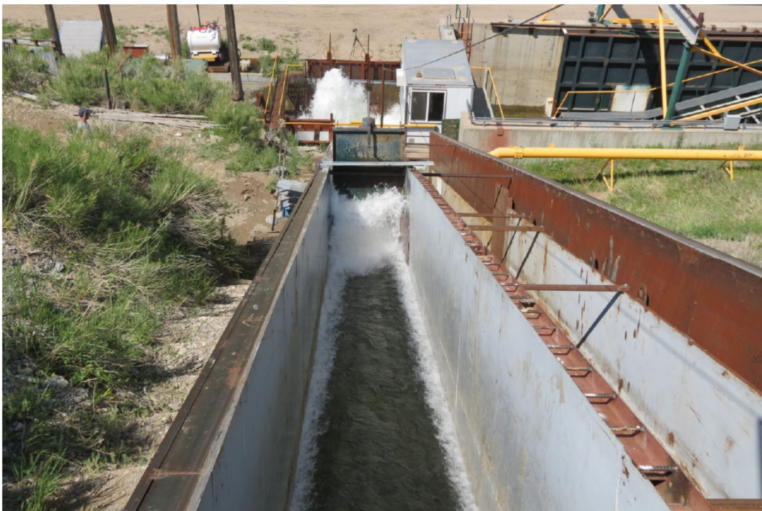
Figure 2 – Hydraulic Jump flume test in progress Shoreblock EPEC SD 475 OCT
