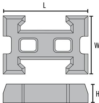
SHORELOC® Concrete unit weight 130-150 lbs./CF, minimum compression strength 4,000 PSI, Maximum Absorption 7% and dimensional tolerance + 1/8".
