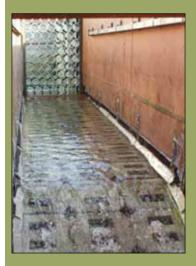
SHOREBLOCK® BD has been successfully tested by Colorado State University, in accordance with the hydraulic performance testing protocol established by the U.S. Federal Highway Administration.
