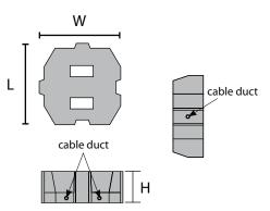
SHOREBLOCK® BD units are manufactured in accordance with ASTM C90, C140 and D6684-04 and the following criteria: concrete unit weight 130-150 lbs./CF, minimum compression strength 4,000 PSI, Maximum Absorption 7% and dimensional tolerance + 1/8".
