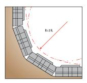
Each block is interconnected by flexible cables, providing articulation between adjacent blocks.
