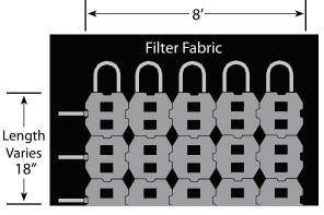
Woven monofilaments are preferred over nonwoven geotextiles because of their high hydraulic conductivity and durability. The soil's particle size (among other factors) will ultimately determine the fabric selection.
