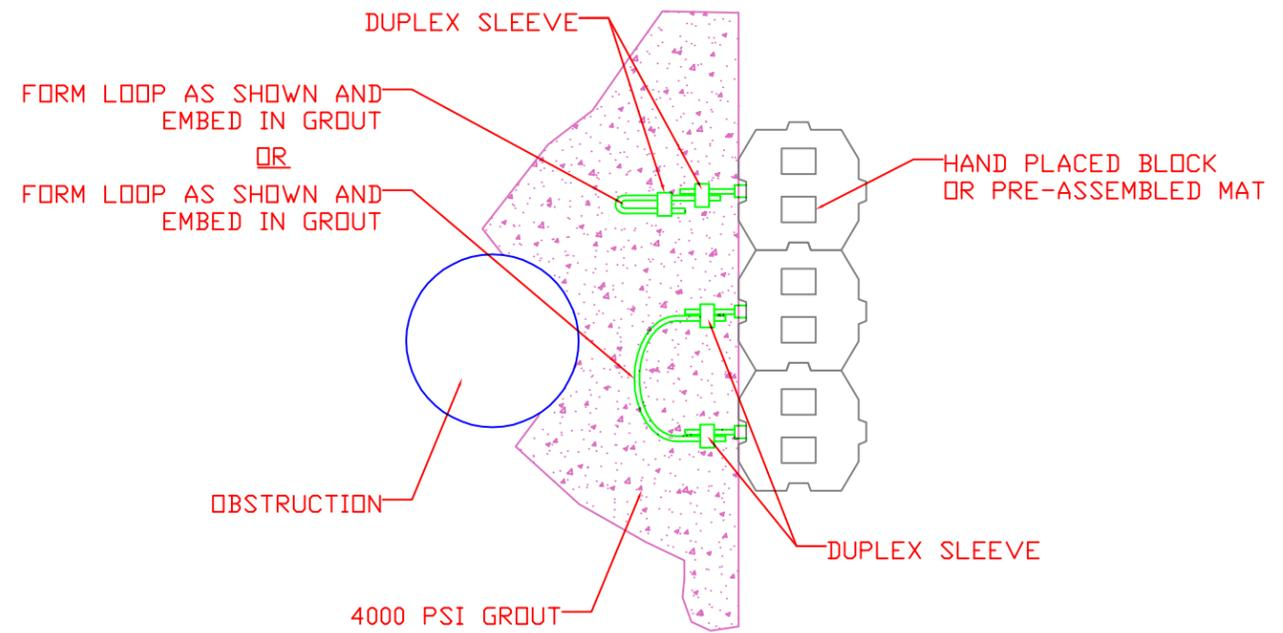
LATERAL CABLE CONNECTION TO GROUT
